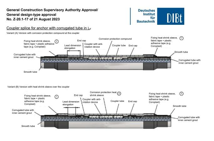
Coupler splice for anchor with heat shrink sleeve in Ltf
