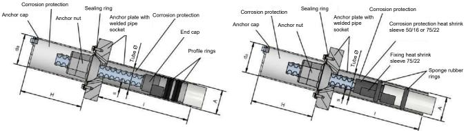
Anchor head with plastic cap for anchor head with corrugated tube and anchor with heat shrink sleeve in Ltf
