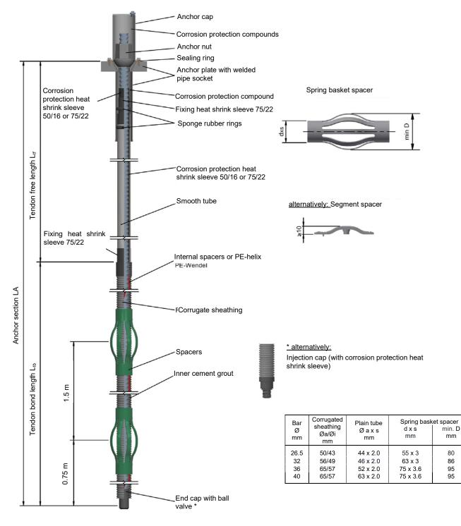
DYWIDAG permanent anchor (single bar anchor) for soil and rock with steel tendons made of: St 950/1050 Ø 26.5 mm, Ø 32.0 mm, Ø 36.0 mm and Ø 40.0 mm Annex 2 Overview of installation version DYWIDAG permanent anchor with heat shrink sleeve
