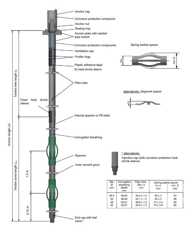
DYWIDAG permanent anchor (single bar anchor) for soil and rock with steel tendons made
