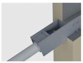
Open top Installation opening for DYNA Grip® Stay Cable Anchorage
