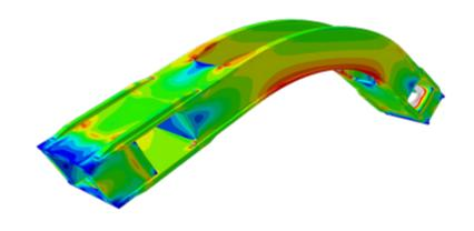
Von Mises stresses of a DYNA® Link Anchor Box with lateral access
