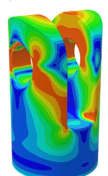
The tests respected an inclination of 0.6° – even towards the inflexible centerline – and an upper load of 0.45 GUTS. They were carried out with a stress range of 200N/mm² at 2 million load cycles.
