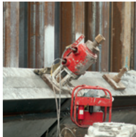
1,500kN jack for T76 temporary anchors
