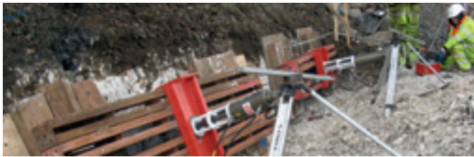
Long Nail/Short Nail testing system for fully grouted hollow bar soil nails
