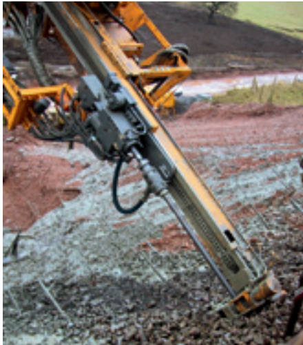
Rotary percussive top hammer (hydraulic)
